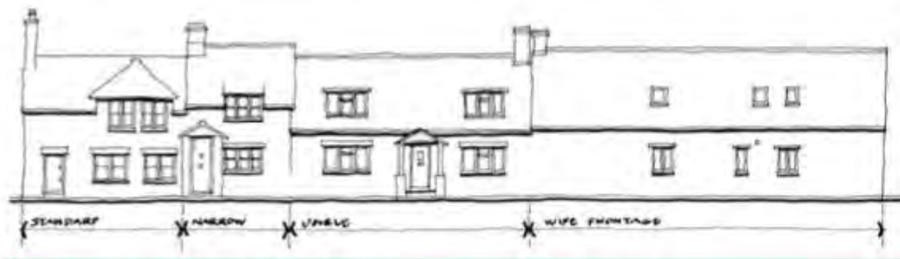
Figure 14: Four cottages – the informal rhythm of the elevations results from a variety in plot widths (North Lane)
